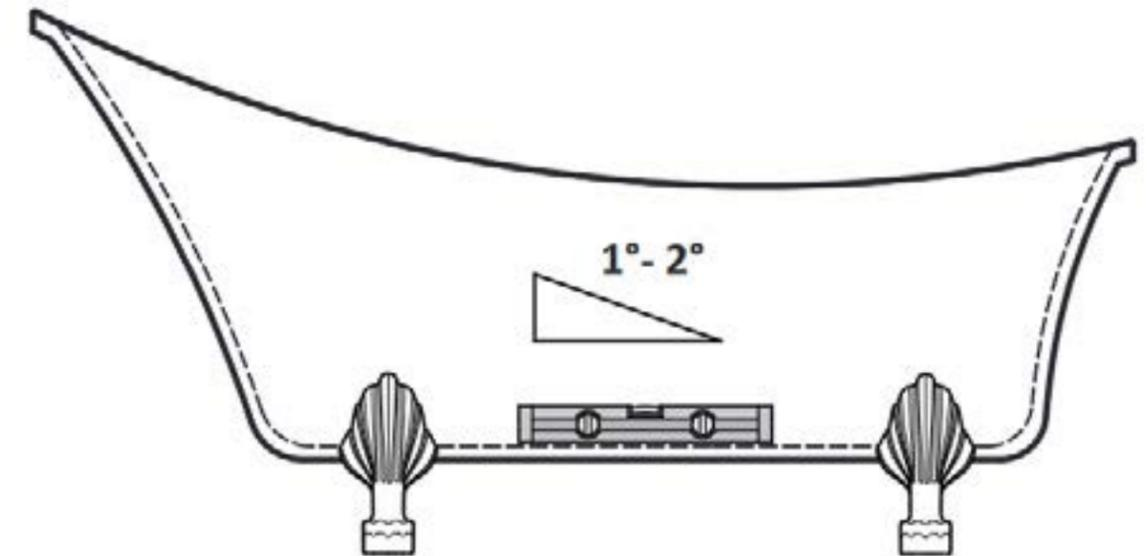
20. Place a level inside the tub. Make sure the bathtub is stable and that all legs rest perfectly on the floor, if not, adjust the leveling pads.
