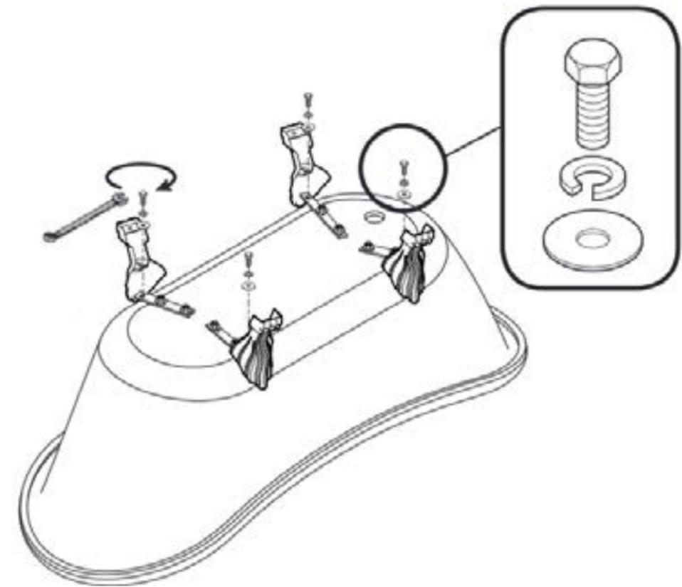
4. Hand tighten the nut so the bar can still slide back and forth in case you have to center it after the feet are installed.
