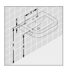
The sink specification sheet will provide the recommended mounting height and show the location of the mounting holes. (The height can be adjusted to your personal preference)
