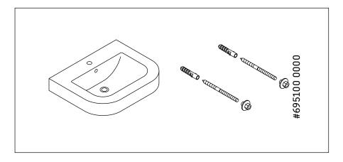
The sink will include mounting hardware model #  $695100\ 0000$ . The plastic anchors provided are for concrete wall applications. For wood stud walls, the lag bolts should be screwed into the wood backing.
