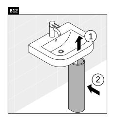
Sently lift the front of the sink to allow pedestal to slide underneath. Slightly loosen mounting if needed to allow for safe lift of basin lip.
