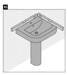
Set sink on pedestal leg carefully, then using a level, properly align the sink.
