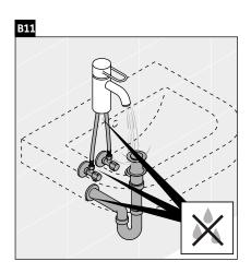
> Test faucet and flush valve to ensure there are no leaks.
