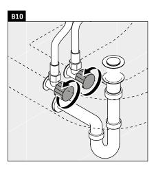
> Turn on shut off valves to test water flow to faucet and flush valve.
