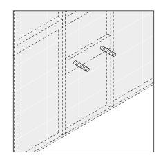
When mounting the sink into a wood stud wall, there must be adequate bracing. We recommend doubling up 2x6's or 2x8's between the studs to form a solid anchoring point. Reference the sink specification sheet to establish the height and the spacing of the mounting bolts.
