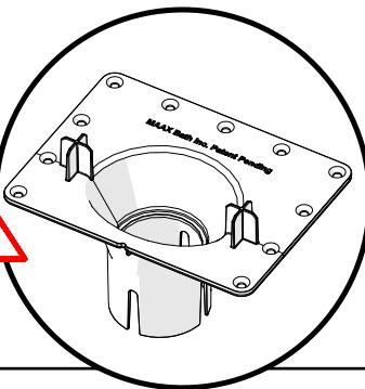
If the optional **F<sup>2</sup> Drain** kit was purchased to facilitate this installation, you have to install it in this step. Please refer to 10032746 installation guide section 1P FS before installing the bathtub.
