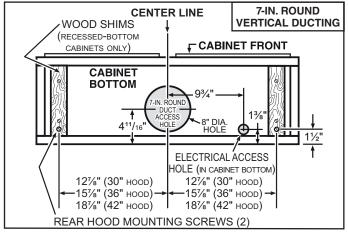
2] Install half-way two (2) ROUND HEAD no. 8 x 5/8" mounting screws into shims/cabinet, according to the proper diagram above, the other 2 ROUND HEAD no. 8 x 5/8" mounting screws will be used later. (Mounting screws are included in parts bag, but wood shims and shim mounting screws are not included.)
