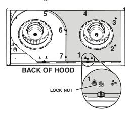
2] Reinstall the blower cover plate (shaded part on illustration above) using the lock nut and the 7 screws previously removed in step 4 on page 10. Pay attention to screw 1 location; from back of hood point of view, it must be located on left side of the lock nut (see inset).
