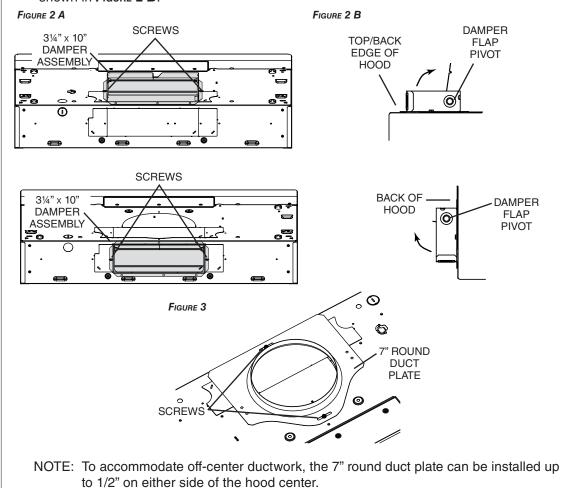
**TIP**: Insert a small length of duct over the 3½" x 10" damper assembly (for rectangular ducting) or 7" round (for round ducting) and seal the joint using aluminum foil duct tape to ease connection with the house ductwork.
