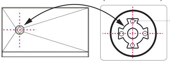
Collar bolts must be lined up correctly to fit the opening in the base
