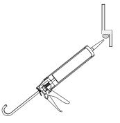
**C.** Silicone underside of Z-molding
