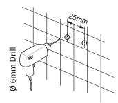
$\ensuremath{\mathrm{B}}$  . insert the wall plugs inside the holes
