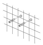
$\ensuremath{\mathbb{C}}$  . Tighten the screws to the wall with wall mounting brackets
