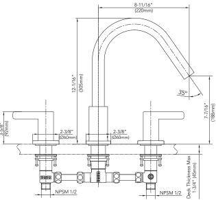
NOTE: Unit for dimensions = inches Dimension in ( ) is mm.
